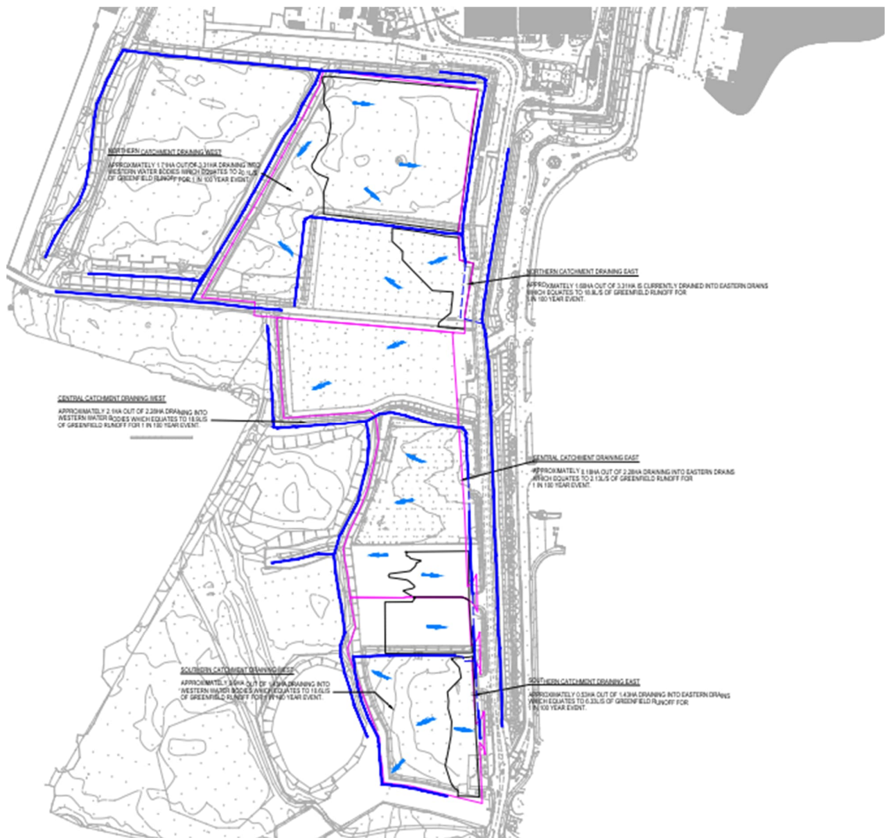
Figure 2-2: Existing Drainage Catchment
